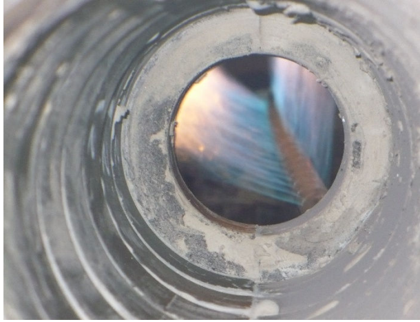
Fig. 1. Ignition via lances. View through the sight glass.
