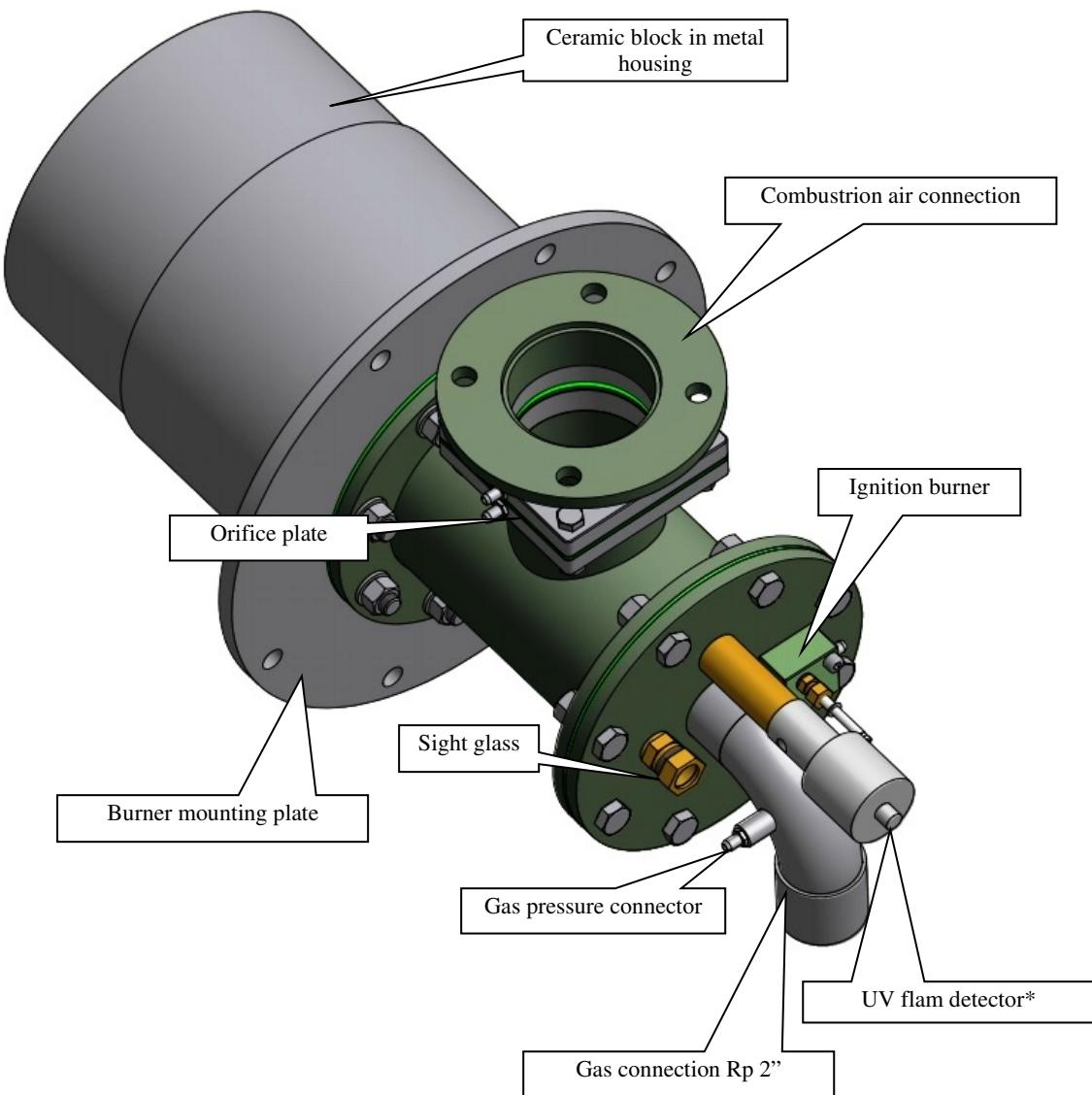
\* In burners operating in continuous-operation furnaces at temperatures below 750°C, the UV flame detector is equipped with a shutter used to verify the correctness of its operation..
