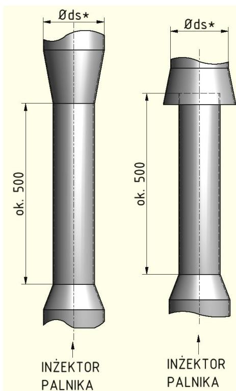
\* selection of the flue gas discharge pipe diameter ( $\phi$  ds) must be consulted each time with PTC PIECOSERWIS.
